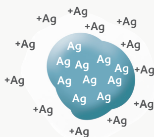
As the water-soluble phosphate dissolves, ionic silver becomes active.
